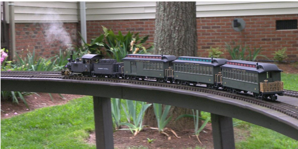
Below left: Ernie Noah's smart, little 0-6-0 is building pressure for an early run. Running a small fan above the stack creates draft for the fire and helps the water to heat up quicker. Ernie scratch-builds a lot of his own equipment, and his work is remarkable.
