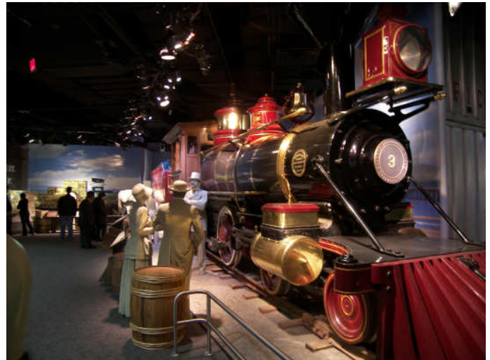
Santa Cruz Railroad Company No 3, named "Jupiter" is a narrow gauge 4-4-0 built by Baldwin in 1876 and formerly on display in the Arts and Industry Museum. Here, No 3 is a scene prop for the westward expansion story.
