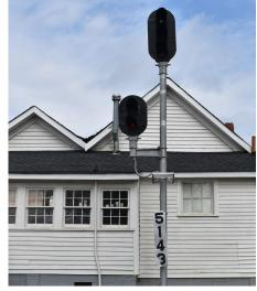
"This project started several months ago, when Jim Alexander gave me a "new" number 3 to replace the damaged one that was on the signal. He received it from Peter Lewis. I later replaced the broken '3' with the new one, but noted it and the other numbers on the signal needed a new paint job.
